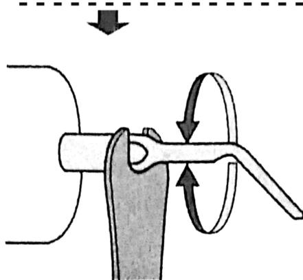
Rotate the head counter clockwise with a wrench to separate the working tip and complete the disassembly.
